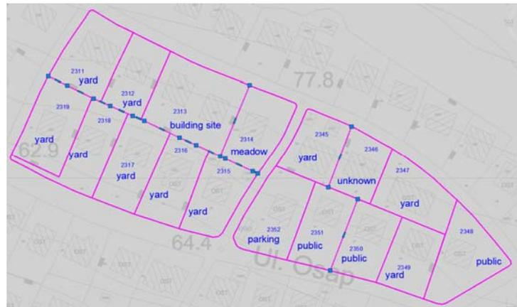
Parcel boundaries are not completely correct. In blue circles there are inconsistencies. Parcel is not 100% closed. During the automatic polygonization – conversion of lines to closed polylines it is possible to define degree of error. Program will automatically correct errors.
